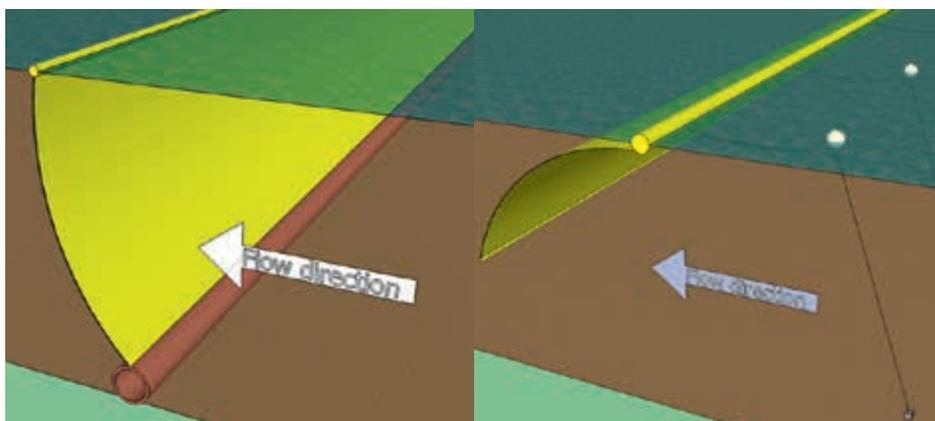
Figure 1. Standing (left) and hanging (right) silt screens.
