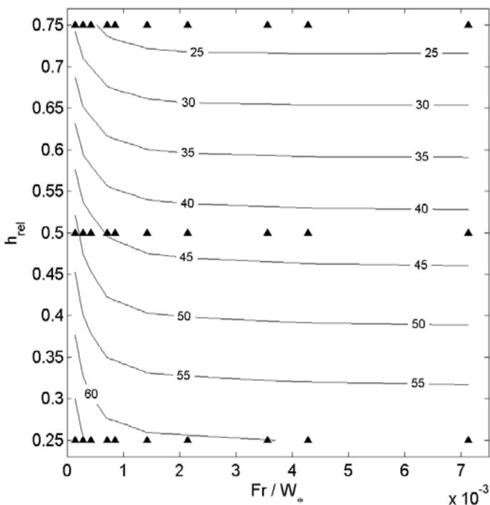
Figure 8. Relative discharge [%] as a function of relative screen height and Froude number over relative screen width.
