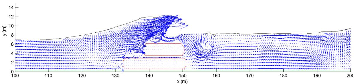
**Figure 2: Wave Modeling for Assessing Wave-Structure Interaction and Stability of a low crested SFC Structure**
